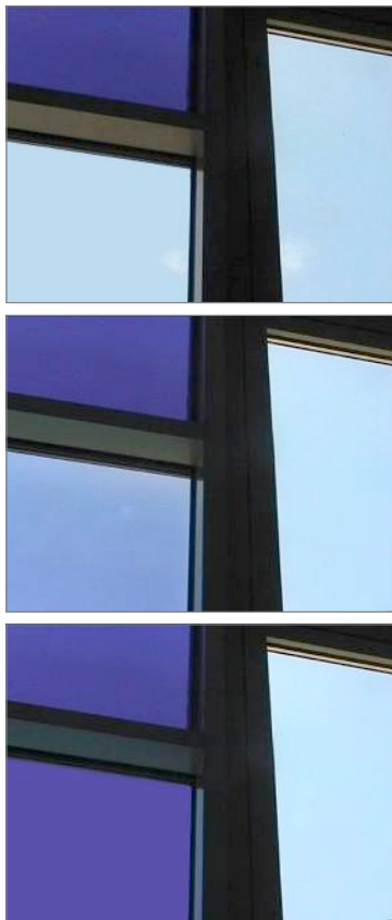
Pictured above are gasochromic windows at varying levels of solar transmittance, and to the right is a schematic of electrochromic and gasochromic technologies. Source: FraunhoferISE.
